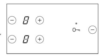
When the cook top is activated (at least one cooking area is activated) you can activate other cooking areas by pressing + or – buttons. Crease or increase heat by using + or – buttons.
